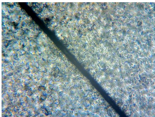
10um line on sapphire substrate
